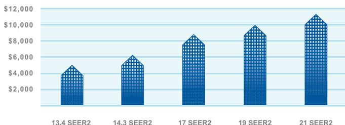
**Note:** Figures represent savings compared to three-ton 10 SEER equipment over 20-year average lifespan, at \$0.14/kWh. National average of unit operation is 2,100 hours. Operating costs vary depending on climate conditions, home characteristics, energy rates and usage patterns. Savings not guaranteed.
