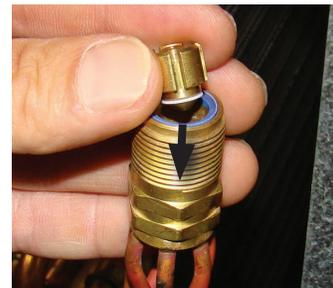
6. Replace the piston with one of the correct size. Do not force the new piston into the body. Make sure the piston moves freely in body.
